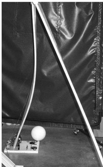
Fig. 23 Joined wing: test article under a 1200 lb load.
